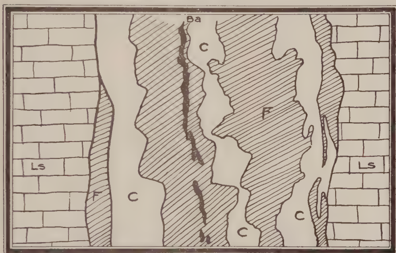
(36) Section at a face in Moore mine (Faircloth) showing relations of minerals and typical vein structure. F. fluor spar; c. calcite; Ba, barite (black); Ls. limestone walls
